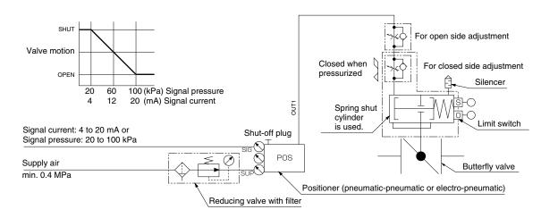
→Butterfly valve closes when air supply fails
